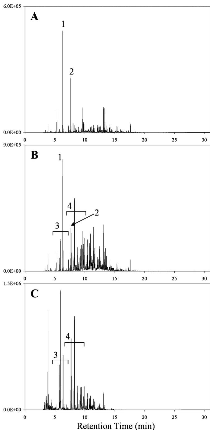
FIG. 5—Chromatograms of (A) heavily burned carpet, (B) gasoline 1 spiked onto carpet then heavily burned, and (C) neat gasoline 1. Major components are labeled: (1) styrene, (2) benzaldehyde, (3)  $C_2$ -alkylbenzenes, and (4)  $C_3$ -alkylbenzenes.
