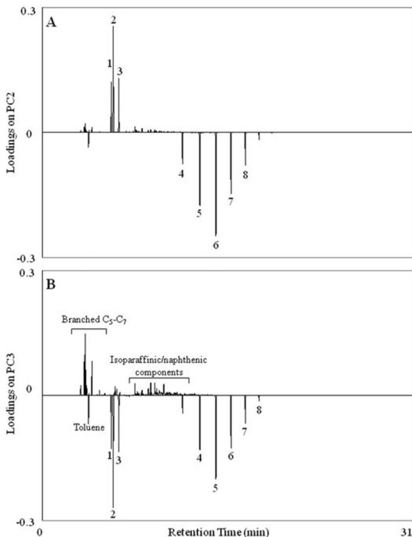
FIG. 8—Loadings plots for (A) PC2 and (B) PC3 for 12 ignitable liquids and six ignitable liquid residues in the presence of increased matrix interferences. Major components are labeled: (1) ethylbenzene, (2) *o*-xylene, (3) *p*-xylene, (4) C<sub>12</sub>, (5) C<sub>13</sub>, (6) C<sub>14</sub>, (7) C<sub>15</sub>, and (8) C<sub>16</sub>.
