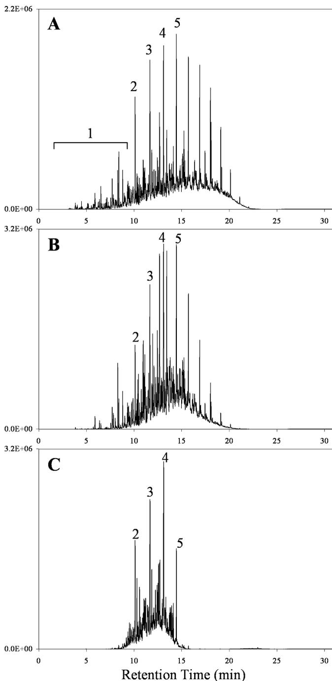
FIG. 4—Chromatograms of (A) neat diesel, (B) diesel ignitable liquid residues, and (C) neat torch fuel, illustrating the similar chemical composition between the ignitable liquids. Major components are labeled: (1) aromatic components, (2)  $C_{11}$ , (3)  $C_{12}$ , (4)  $C_{13}$ , and (5)  $C_{14}$ .
