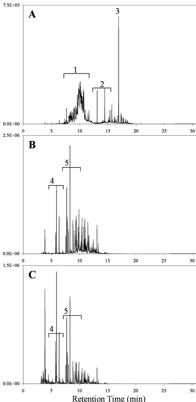
FIG. 1—Chromatograms of (A) lightly burned carpet, (B) gasoline 1 spiked onto carpet then lightly burned, and (C) neat gasoline 1. Major components are labeled: (1)  $C_{11}$ – $C_{12}$  isoparaffinic/naphthenic components, (2)  $C_{13}$ ,  $C_{14}$  normal alkanes, (3) diester related to adipic acid, (4)  $C_2$ -alkylbenzenes, and (5)  $C_3$ -alkylbenzenes.
