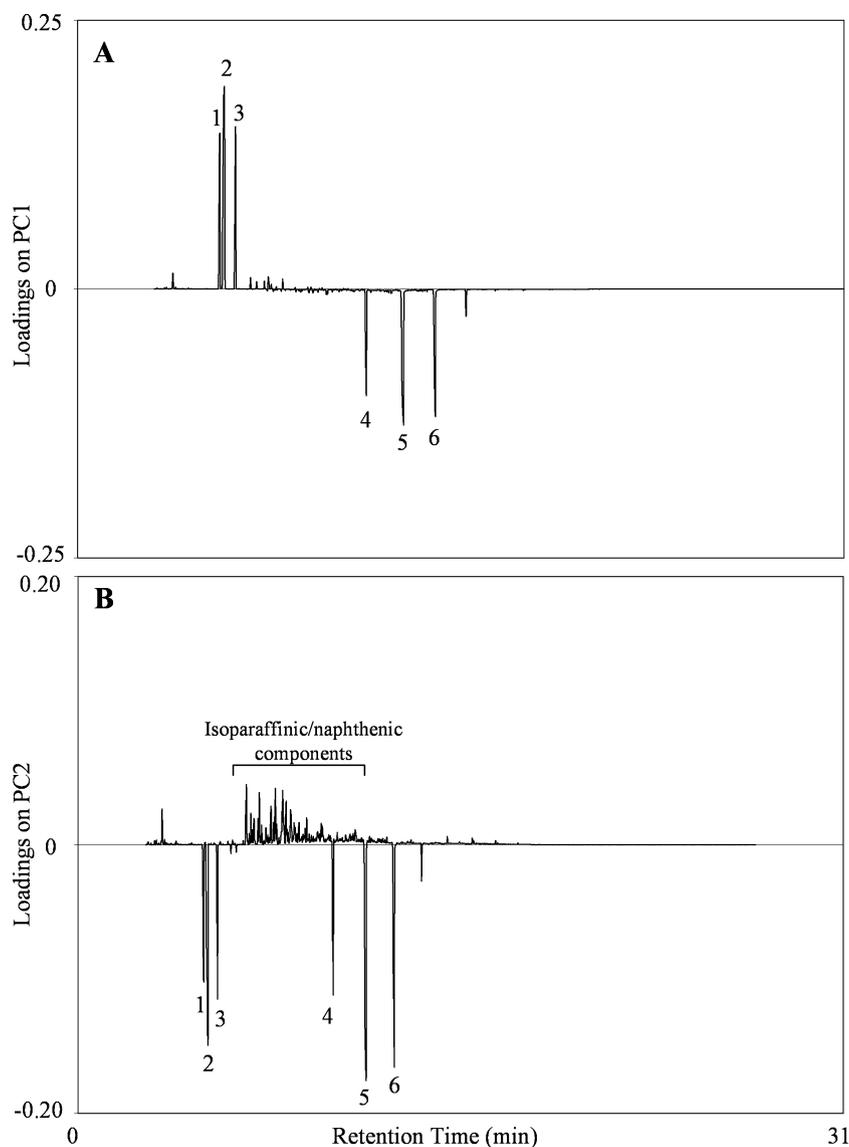
FIG. 3—Loadings plots for (A) PC1 and (B) PC2 for six ignitable liquids and the corresponding ignitable liquid residues in the presence of minimal matrix interferences. Major components are labeled: (1) ethylbenzene, (2) *o*-xylene, (3) *p*-xylene, (4)  $C_{12}$ , (5)  $C_{13}$ , and (6)  $C_{14}$ .
